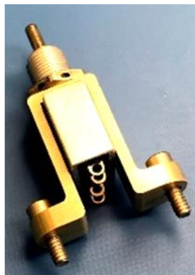
Attach screws to Separation Switch
