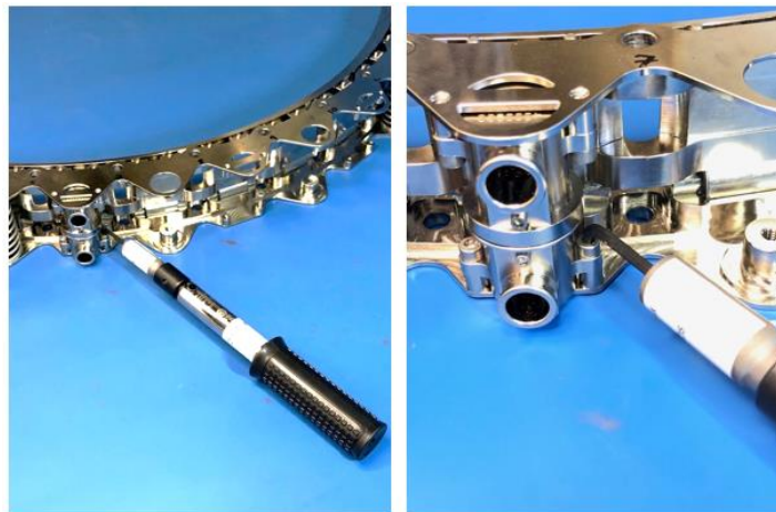
Figure 11-7: Separation Connector attachment torque
