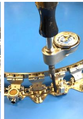
Tighten screws with Torque Wrench
