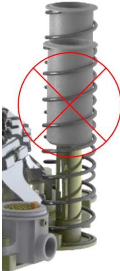
Figure 7-4: Do not use Springs to rotate ALB
