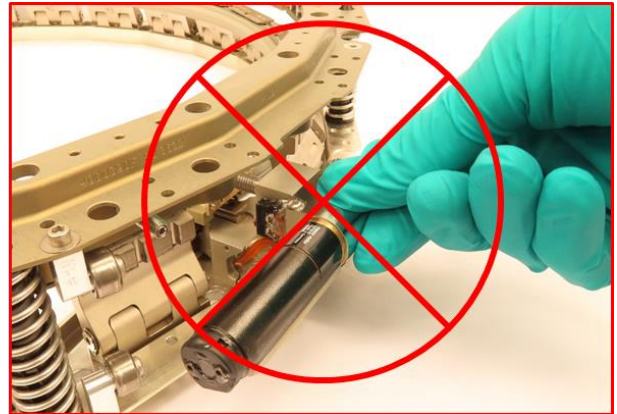
Figure 6-4: Do not touch the gear cover
