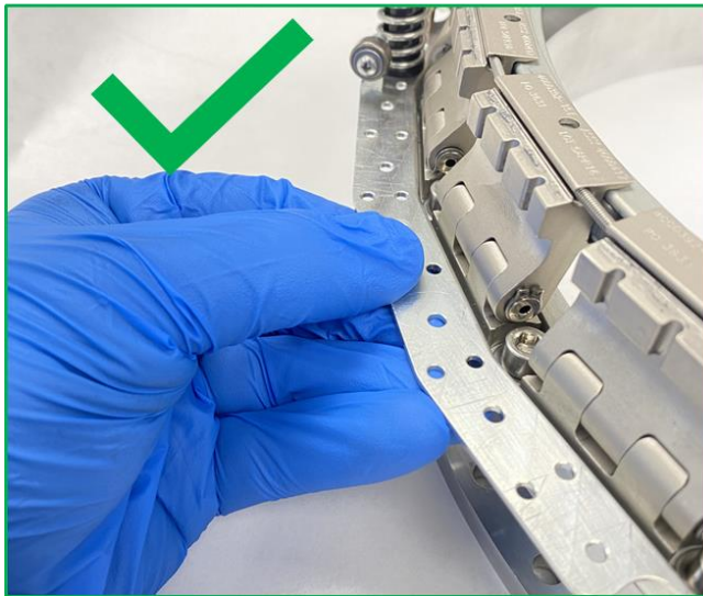
Figure 6-9: Uses flanges to handle the Lightband
