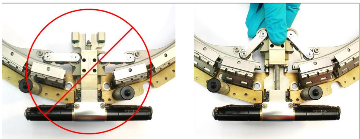
Figure 8-2: Verifying pre-Mate Sliding Tube position
