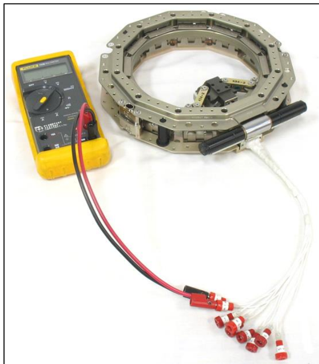
Figure 16-2: DMM and DE-9 breakout cable used to measure Motor Bracket Assembly resistance.
