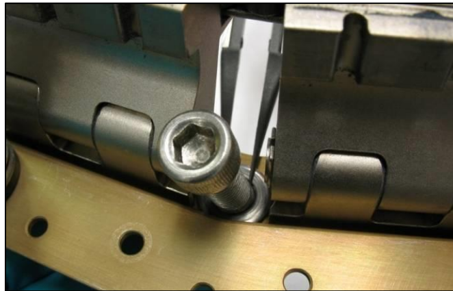
Figure 12-1: Removing a SHC screw from the Lower Ring, outer view
