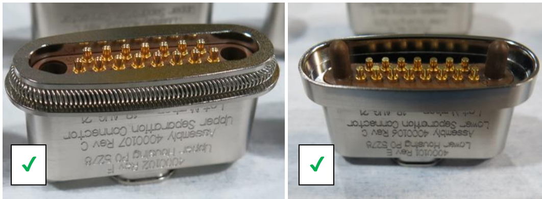
Figure 8-7: Examples of Pristine Upper and Lower Connectors with properly installed matrices.
