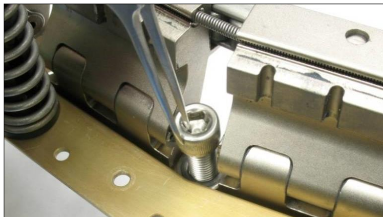
Figure 7-2: Inserting a SHC screw between Leaves on Lower Ring.
