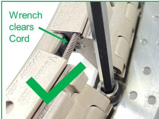
Figure 6-6: Ensure the Leaf Retaining Cord is not contacted
