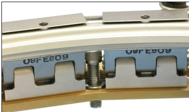
Figure 12-1: Removing a SHC screw from the Lower Ring, outer view
