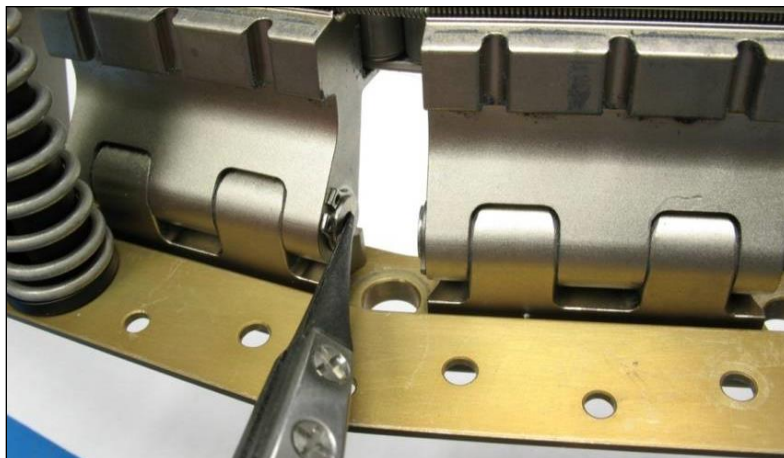
Figure 7-1: Pushing Leaf Pin to side to make room for SHC screw (15.000-24 only).
