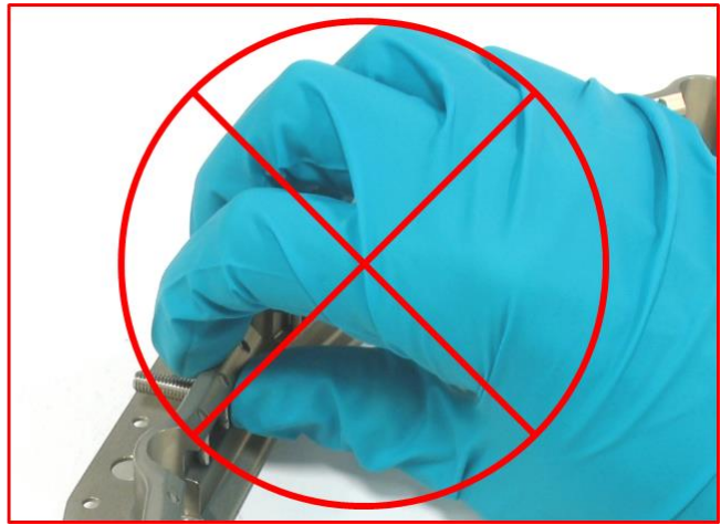
Figure 6-2: Do not touch the Leaf lip or its corresponding groove in the Upper Ring
