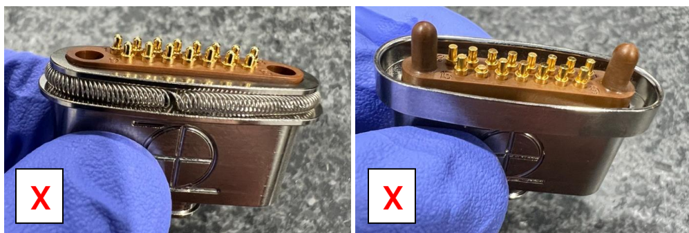
Figure 8-6: Examples of Upper and Lower Connectors – damaged and poorly assembled.
