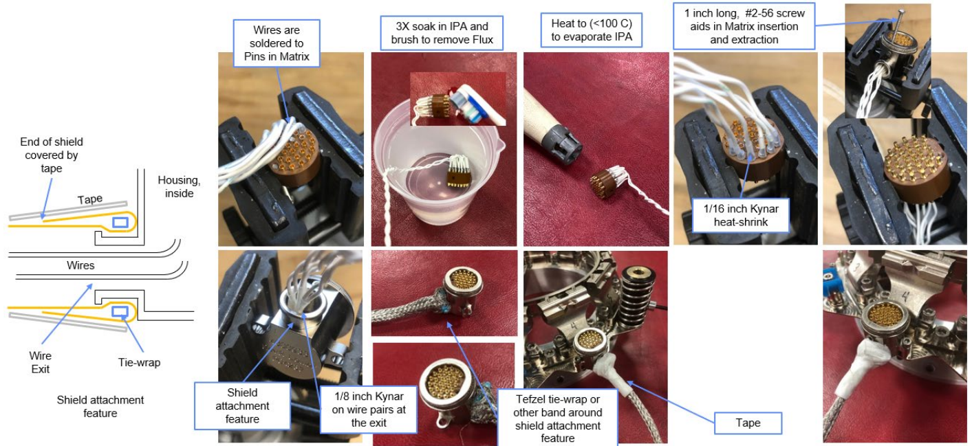
Figure 15-5: Wiring of Separation Connector
