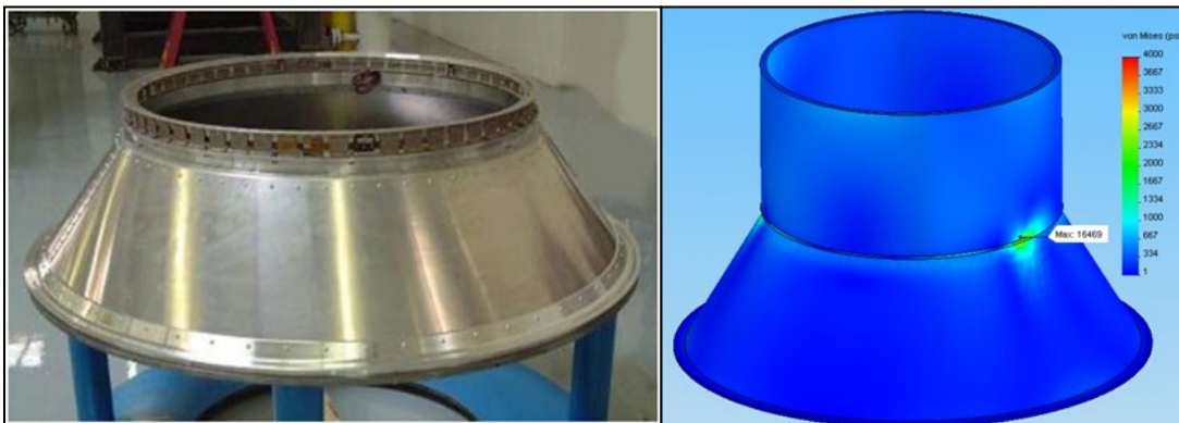
Figure 4-12: An MLB attached to a launch vehicle cone and CAD model showing resulting stress peaking that occurs when adjoining two warped surfaces
