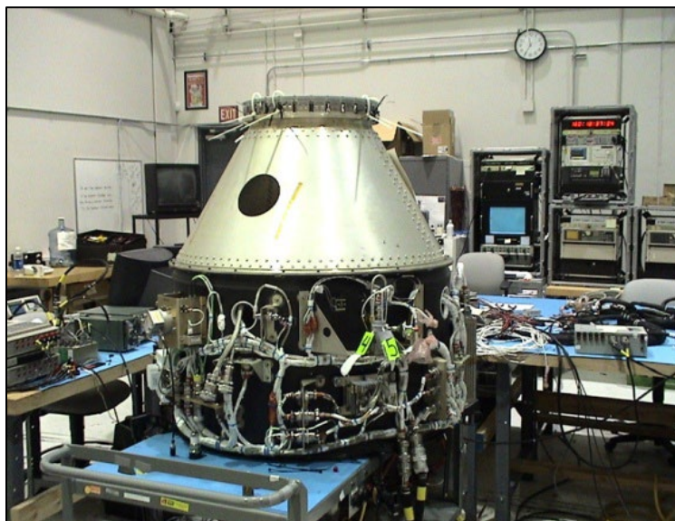
Figure 11-1: Electro-mechanical fit check and a separation test
