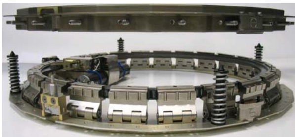
Figure 2. A separation system: The Lightband
