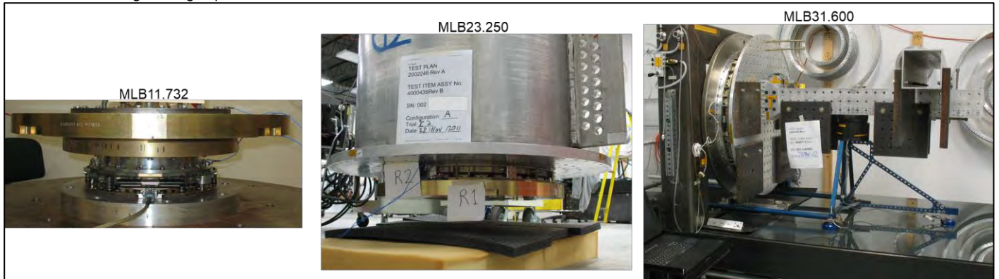
Figure 10-3: Test configurations for MLB generated shock
