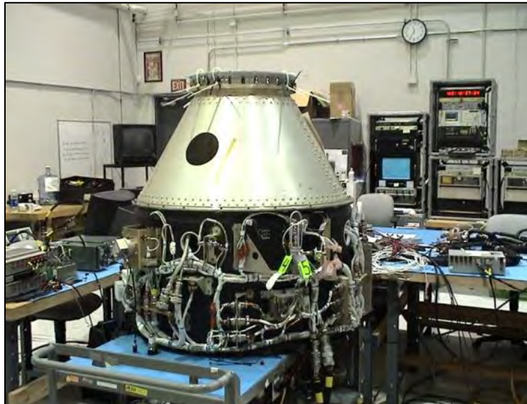
Figure 21-1: Electro-mechanical fit check and a separation test with an MLB
