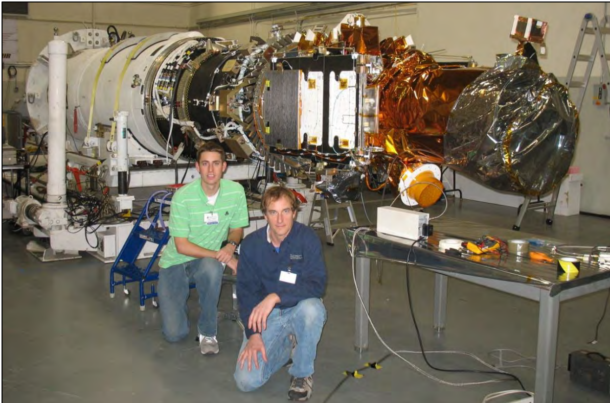
Figure 15-2: PSC engineers perform a horizontal integration (with an isolation system) of a space vehicle onto a launch vehicle
